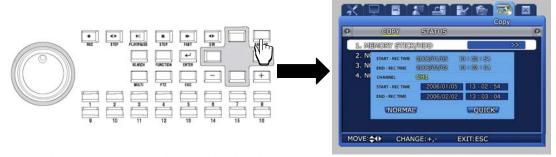
After selecting a storage medium, select the channel for which COPY will be carried out and the i mage information [START-REC TIME /END-REC TIME]. After a selection is made between NO RMAL COPY and QUICK COPY, COPY is started.
